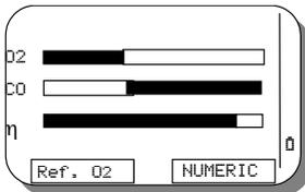
Using GasConfig Software, you can program the graph page: Assign up to 6 different parameter, range and increment direction. See chapter 9 for software instructions.
