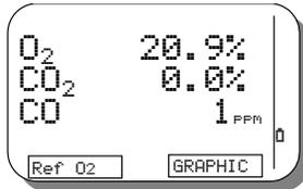
If the graphical option (Table E=4 on ordering code) is installed, the instrument can display the measured values as bar-graph. Press the **[GRAPHIC] (F2)** key to change mode.
