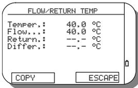
On the “Measure” field, the instrument will display the current temperature value measured using the connected thermocouple. The error message “Tc open” will be displayed if the thermocouple is not connected or broken. Positioning the thermocouple on the flow pipe.
