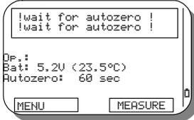
This page displays the following information: operator name, battery charge level, instrument internal temperature and the seconds to end the autozero procedure.
