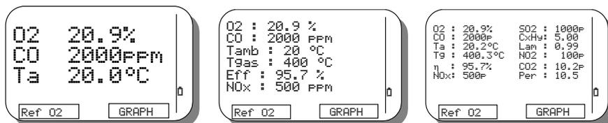
Two boxes are positioned on the bottom of the display. They contain the name of the function assigned to the [F1] and [F2] function keys.
