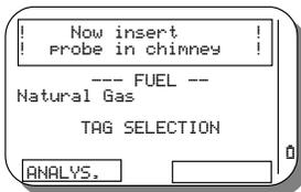
This page allows the operator to change the fuel used and to select the Tag between the available.
