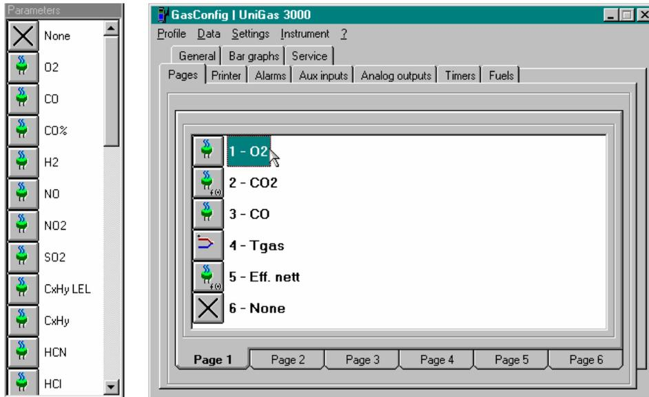
The window on the left is an icon list. This list shows all possible parameters that are possible to visualize on the analyzer (O<sub>2</sub>, CO, T<sub>gas</sub>, Draught, etc.).
