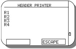
Select the R1, R2, R3, and R4 rows and press **[ENTER]** to insert or change the text. Press **[ESCAPE]** (F2) to return to the previous page.
