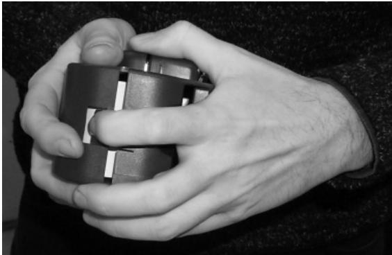
Extract the exhausted paper roll. You can use standard paper roll but you have to check before for its dimensions (max. 57mm  $\pm$ 1mm large and 48mm  $\pm$ 1mm roll diameter).
