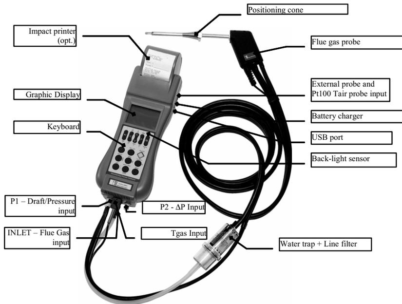
At the bottom of **EGA4** you can see all sampling probe connectors: gas inlet, pressure and draught input, thermocouple input for gas measurement and the 2<sup>nd</sup> pressure inlet connector.
