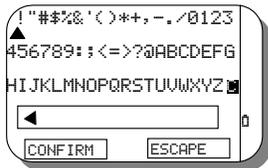
A "▲" symbol below the " " (blank) character in figure, represent the cursor. It is used to identify the selected character; you can move it using the [◀], [▶], [▲] and [▼] keys. The box below the characters table shows the currently inserted text. The symbol "◀" is the end of line symbol.
