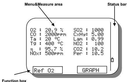
The Menu and Measure area displays the analysis data, the menu and all messages for the operator. The measured and calculated parameters are displayed in different pages of 6 parameters each.
