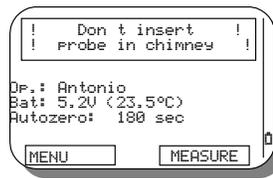
2. Select the combustible used by burner. It is possible choosing between 4 preset and other 6 customizable types.
