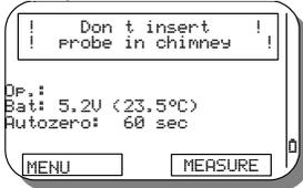
if the optional Autozero valve option is installed, the display will show the page below:
