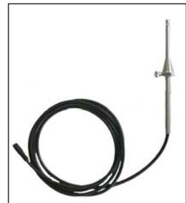
It is important to measure the true combustion air temperature to have a correct boiler efficiency computation. The EGA4 has a auxiliary Rtd input to measure simultaneously the air temperature. A Pt100 with a 6 meters long cable can be connected on the right side of the analyzer.
